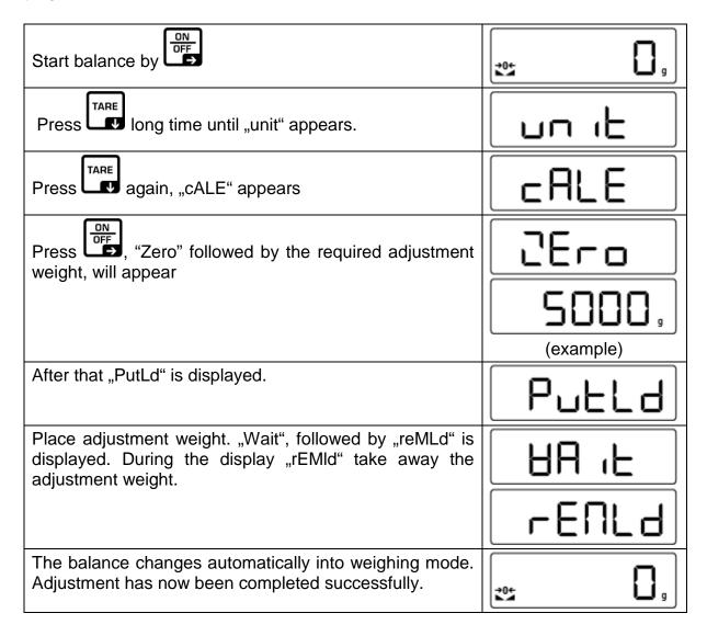
If an adjustment error occurs or a wrong adjustment weight is placed, "WronG" is displayed. Repeat adjustment.
